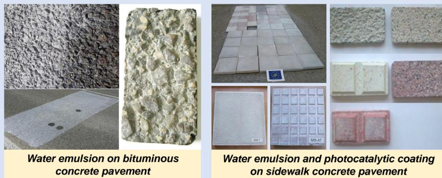
Water emulsion on bituminous concrete pavement
