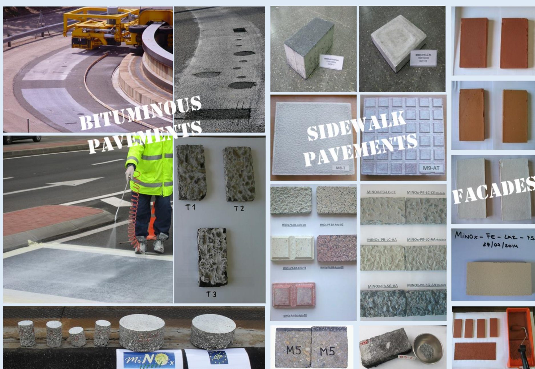
Some photocatalytic materials tested to prove their NO removal capacity
