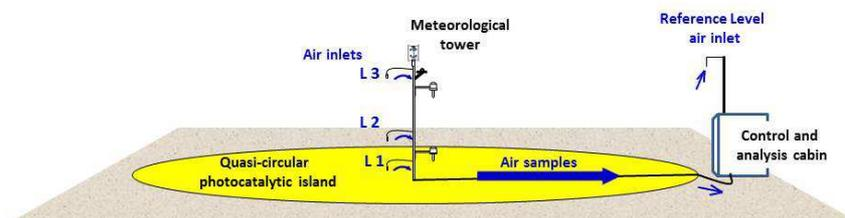
**Fig. 1.** Experimental platform at CIEMAT.
