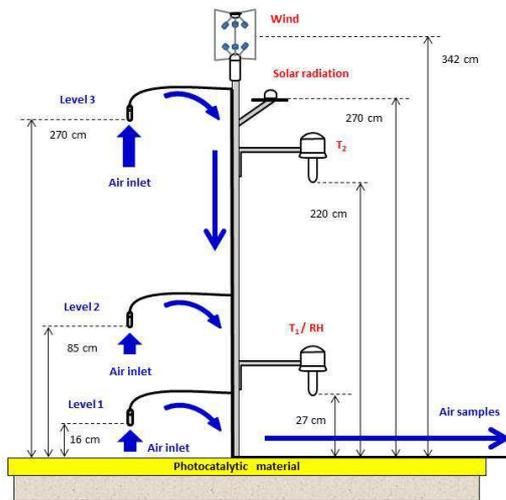
**Fig. 2** Scheme of the mast with meteorological sensors and probes for measuring ambient air.
