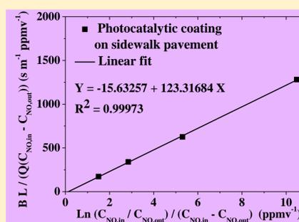
By employing the equation (3) and the experimental data under variable NO inlet concentration (100 to 1000 ppbv), the Langmuir-Hinshelwood kinetic model was used to estimate kinetic parameters (reaction constant,  $k$ , and adsorption equilibrium constant,  $K_{ad}$ ). Following, the deposition velocity,  $v_{ph,NO}$ , which corresponds to the concentration-independent kinetic constant of a first order law of a chemical surface reaction of NO, has been estimated.
