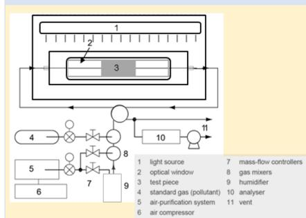
Scheme of the ISO 22197-1 test equipment
